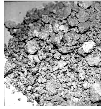
Figure 15: Consistence of the mortar sampled from "incoccio" in pillar 1 of the S. Nicolò Church.
