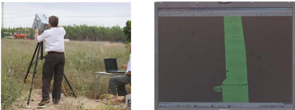
The digital survey is a powerful tool for the structural engineering, but should be complemented with other techniques as the sonic and ultrasonic testing, settlement difference monitoring and others... For example, for the industrial chimney, we have obtained the brick masonry elastic modulus or constant and the inner hollow in the chimney base. These parameters are relevant for the numerical simulation and the later dynamic analysis to get the eigenvalues or natural vibration.
