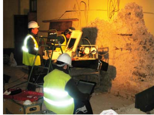
Fig. 6 “Instant during a double flat jack test”
