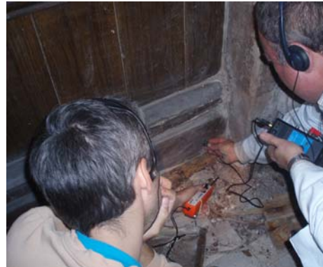
Fig. 21 "Sonic methods for the determination of activity of the hypothetical bodies xylophages"
