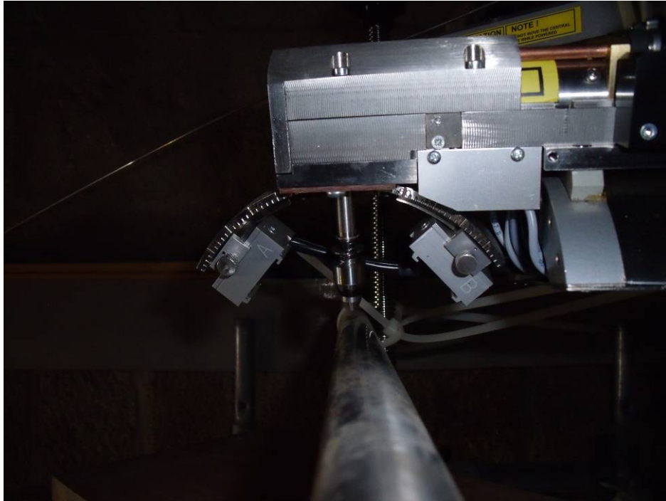
Fig. 8 The equipment placed on the bar in the process of measure
